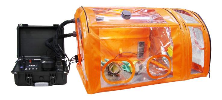
The glove box is intended to protect the operator and the environment from contamination during work with pathogenic biological agents.
